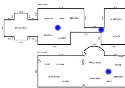
**Example 3:** This is a two-story home with a need for three carbon monoxide detectors since there are two floors as well as two separate sleeping areas upstairs.
