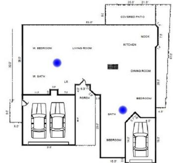
**Example 2:** There are two different sleeping areas in this single story house, so there is a need for two carbon monoxide detectors as indicated by the blue dots.
