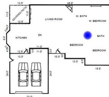
**Example 1:** There is one small hallway connecting all bedrooms in this single story house, so there is only one carbon monoxide detector required as indicated by the blue dot.
