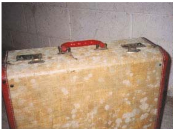
Mold growing on a suitcase stored in a humid basement.
